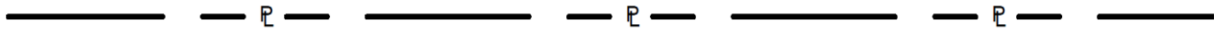
Figure 17: Modified phantom linetype used for survey located street lines and lot lines
